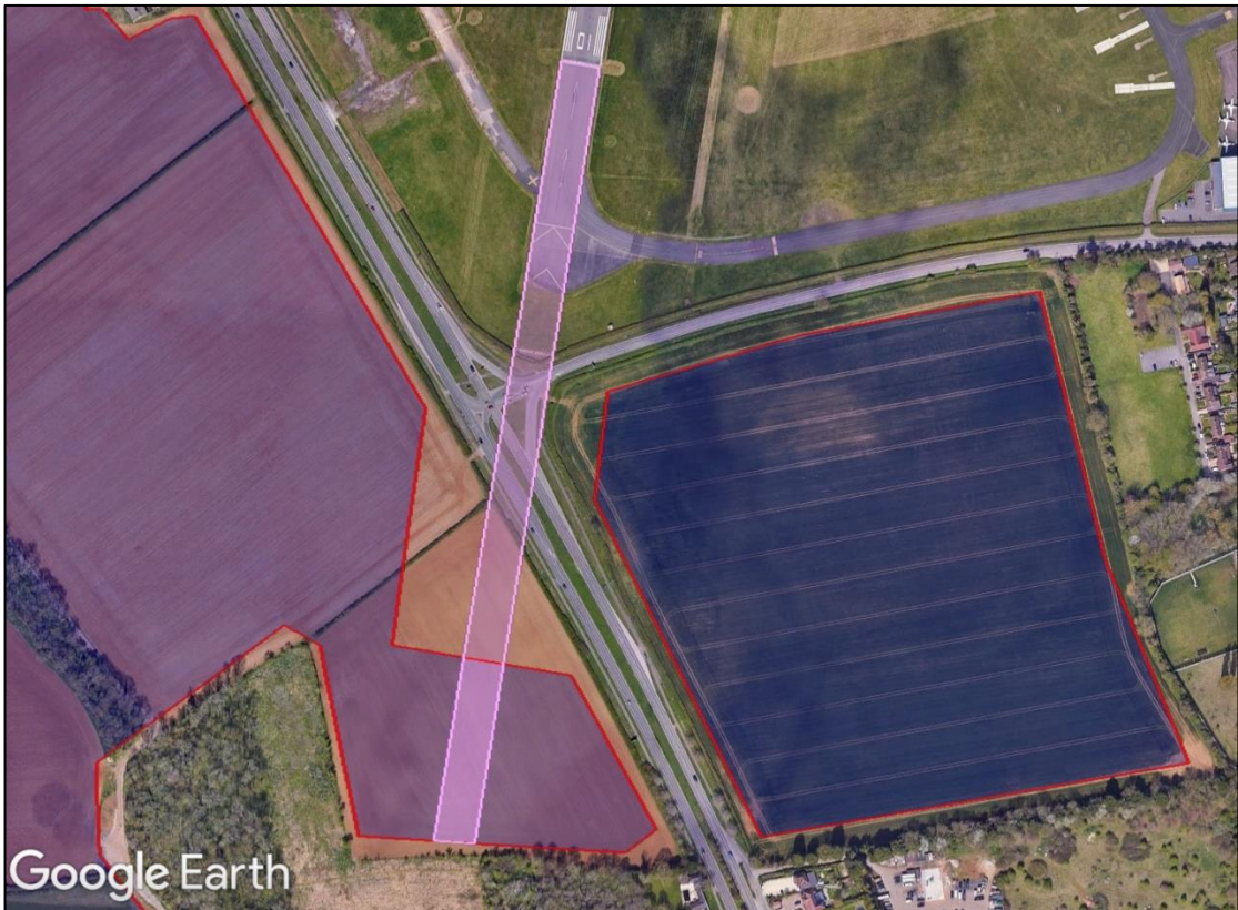
Figure 5 The suggested designated EFATO safeguarded zone, running along the extended runway centreline
